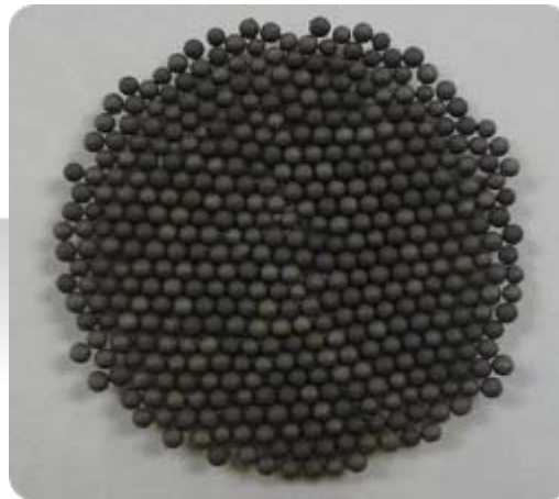
Hollow Shells – SiC (0.24 g/cc)
