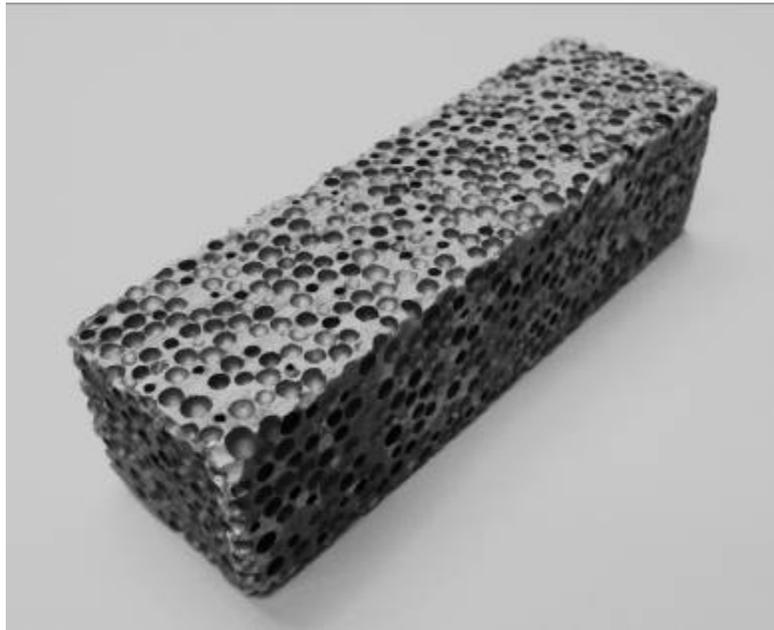
Figure 2 – Prepared Syntactic Foam Test Sample
