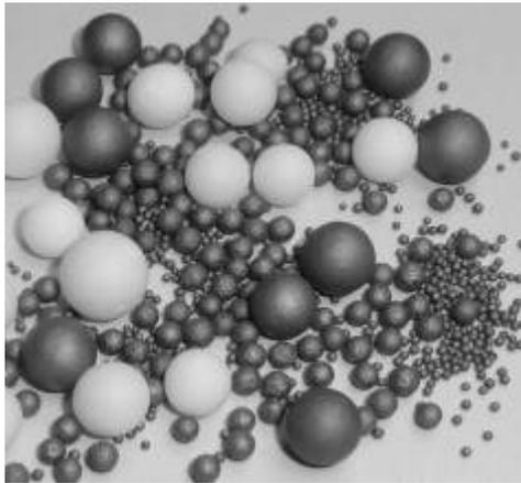
Figure 1 – Hollow shells of various size, density and, material produced by DST.
